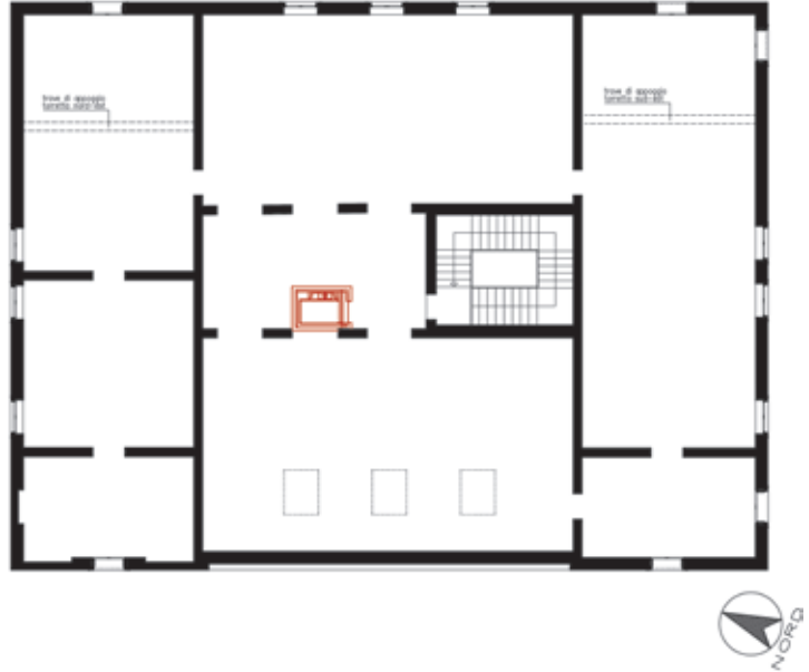
Fig. 11.1 Villa Trissino at Cricoli. Project by A. Pereswet Soltan for lift installation - 2016 Highlighted: 2016 century alterations Attic
